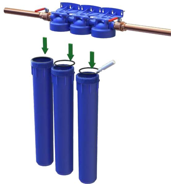
**9** Install the 3 filter in the proper order:
